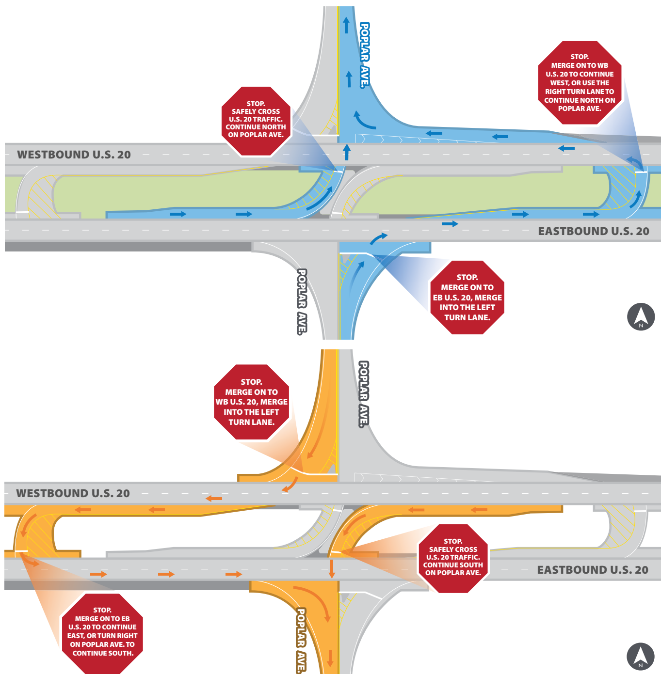
Figure 5.3: Reduced-conflict interchange (Example shows the reduced-conflict interchange at U.S. 20 and Poplar Ave. in Webster County)
