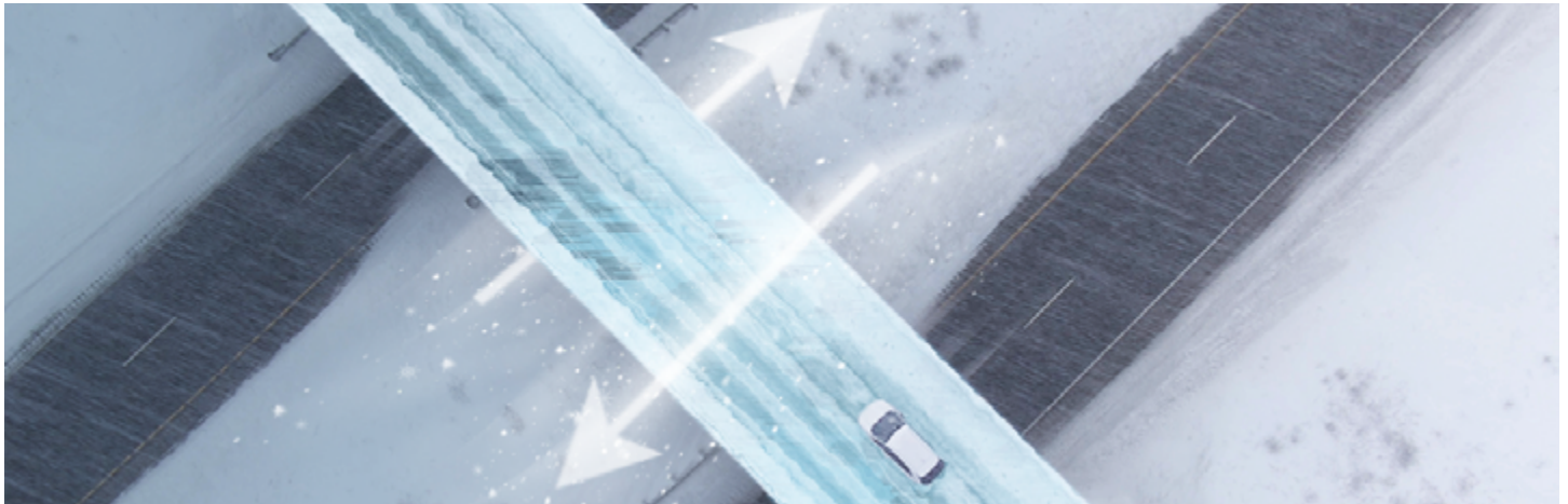
Figure 5.10: Ice forms on bridges first due to circulating air both above and below the road surface.
