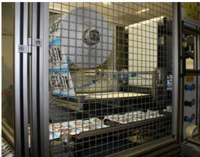
This machine adheres the printed vinyl to metal sheeting during the license plate making process.
