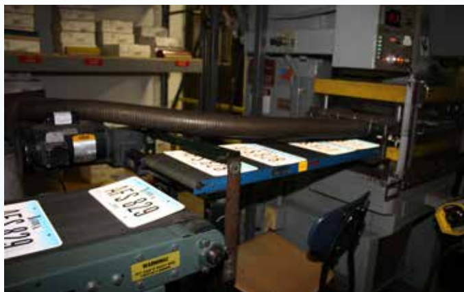
After the vinyl is adhered to the metal sheeting, it is die cut and punched into new license plates.
