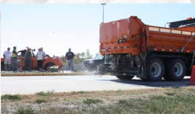
The salt retention study examined the amount of salt retained on the roadway using various spreaders, brine rates and truck speeds.
