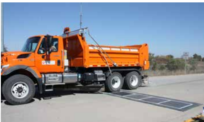
The salt retention study examined the amount of salt retained on the roadway using various spreaders, brine rates and truck speeds.
