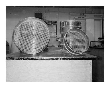
A set of **305 mm (12 in.) Diameter Sieves** may be used for testing fine aggregate or aggregate containing both coarse and fine material.
