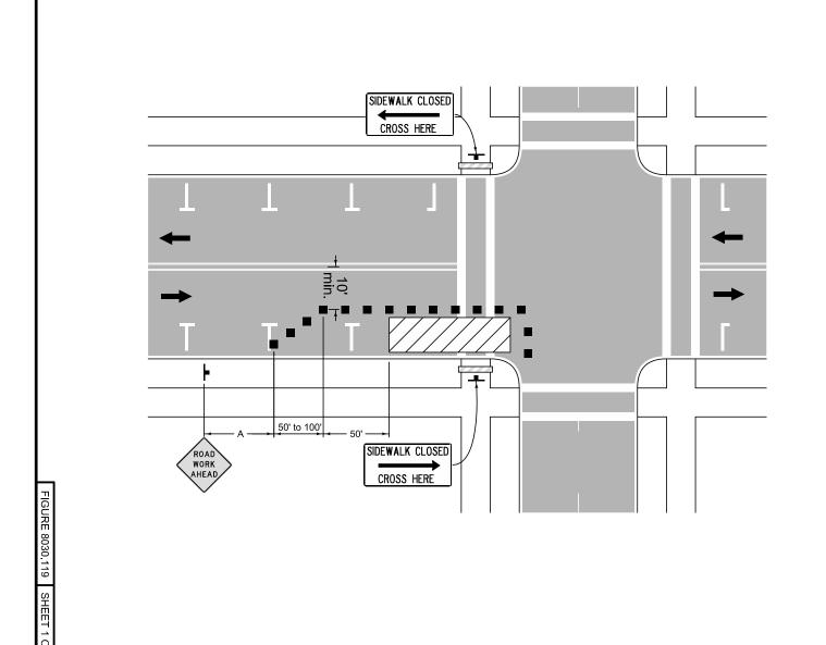
Use when work activities close crosswalk or reduce width to less than 4 feet. Ensure temporary facilities are detectable and include accessibility features consistent with the features present in the existing pedestrian facility.
