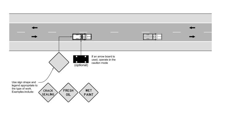
Use for pavement marking and surface maintenance operations in daylight hours only.
