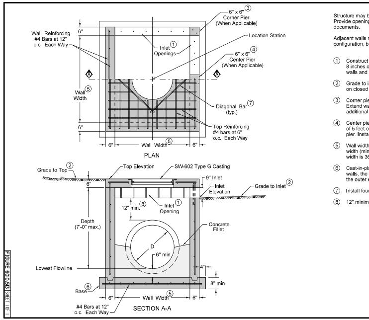
Structure may be built with openings on any or all sides. Provide openings and orientation as specified in the contract documents
