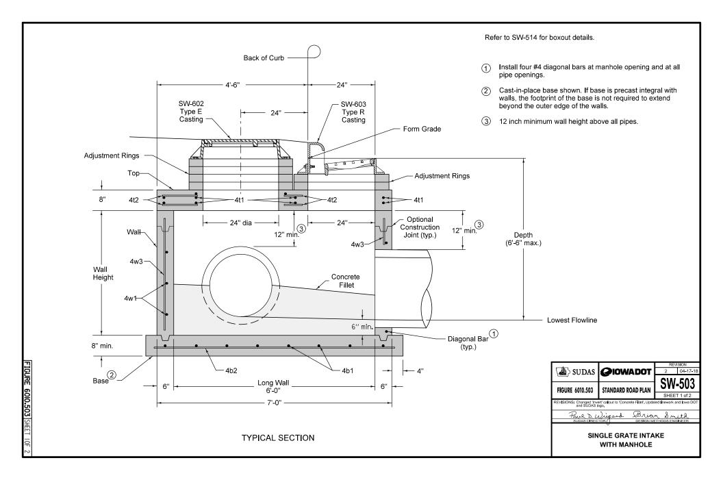
Install four #4 diagonal bars at manhole opening and at all pipe openings.
