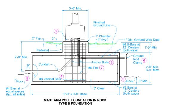
Type B Foundation is applicable for traffic signal poles with mast arm lengths up to 60 feet.
