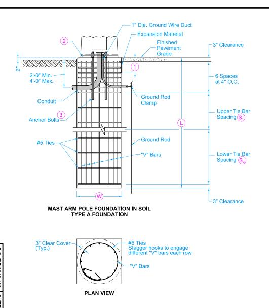
The Type A Foundation is the normally required foundation construction. Where rock is encountered, the Engineer may approve the use of the Type B or C Foundation. Prior to installing a foundation in rock, obtain a subsurface investigation certified by a geotechnical engineer licensed in the State of Iowa.
