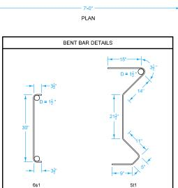
NOTE: ALL DIMENSIONS SHOWN OUT TO OUT. D = PIN DIAMETER
