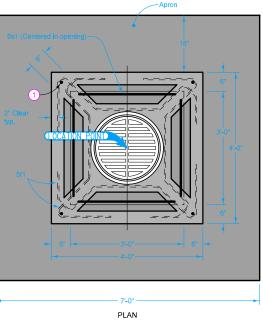
Top of intake may be poured in the field or precast. For precast units, place a 1 inch diameter X 3 inch deep alignment hole 3 inches from each side of the corners of the unit.
