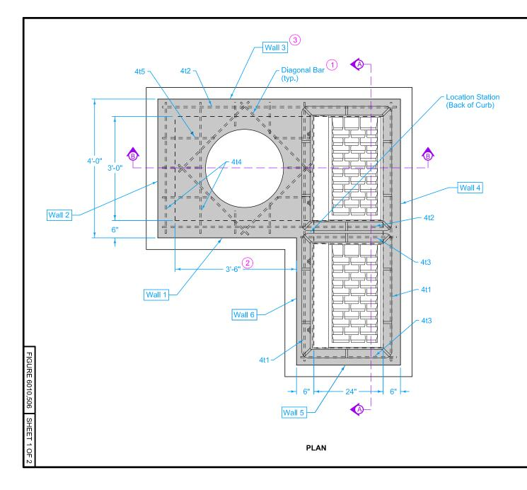
Maximum pipe diameters are set based on maximum structure depth of 6 feet-6 inches and the objective of placement of the centerline of the pipe on the centerline of the manhole opening for maintenance purposes.
