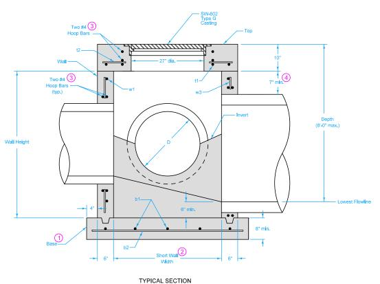
Adjacent walls may have different widths based upon pipe configuration, but structure must be rectangular.
