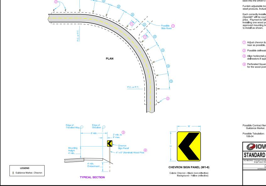
To be effective, Chevron Sign Panels should be visible for at least 500 feet. Attach Chevron Sign Panels to the adjustable brackets at an angle so headlight beams are not reflected back into the driver's eye.
