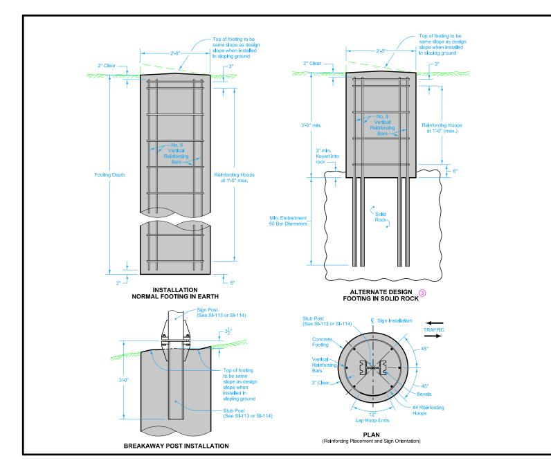
Construct the footing as shown for normal footing in earth. Where solid rock is encountered, the alternate design for footing in solid rock may be used with the approval of the Engineer.
