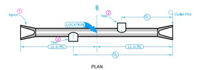
REINFORCED CONCRETE PIPE CULVERT
