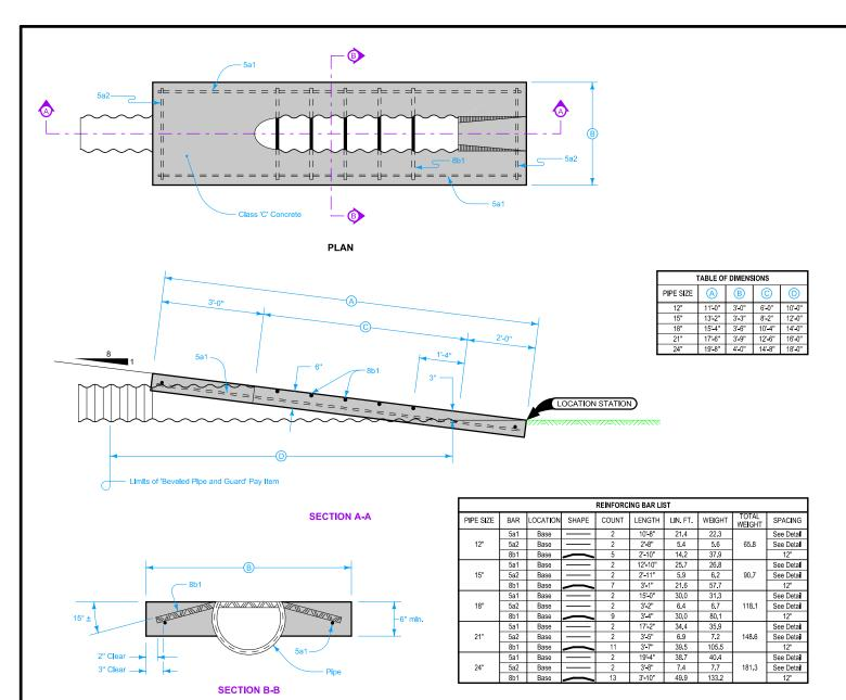
For reinforcing steel used in construction of "Beveled Pipe and Guard", use deformed bars meeting the requirements of Article 4151.03 of the Standard Specifications and hot-dip galvanized according to ASTM A123.
