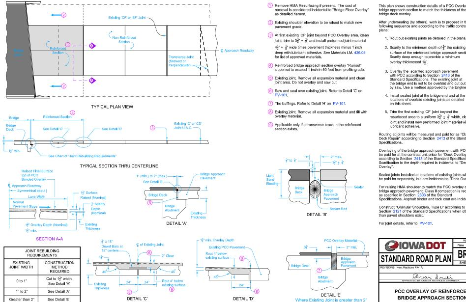
This plan shows construction details of a PCC Overlay on a bridge approach section to match the thickness of the
