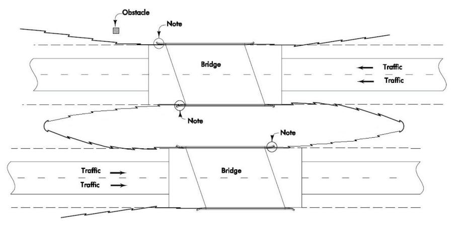
Note: Install Terminal Connector on outside of rail
