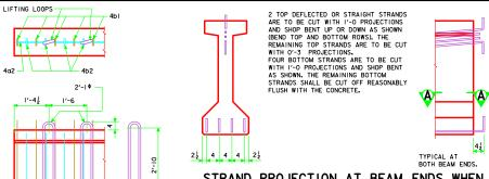
LIFTING LOOP DETAIL ALTERNATE TYPES MAY BE SUBSTITUTED WITH THE APPROVAL OF THE ENGINEER, LIFTING LOOPS ARE TO BE STRUCTURAL GRADE.
