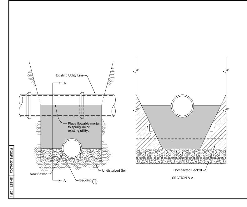
Use flowable mortar utility line support when new utility excavation is crossing under an existing utility line (sewer lines, water lines, gas lines, etc.) as directed by the Engineer.
