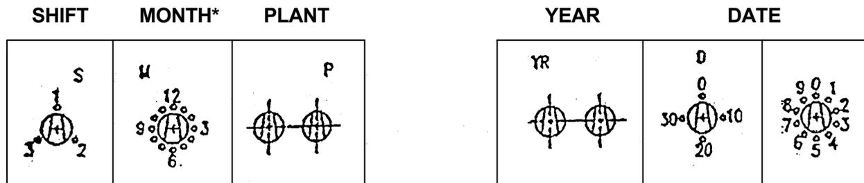
**\*ACTUAL ENCODING ON PIPE DOES NOT INCLUDE NUMBERS**
