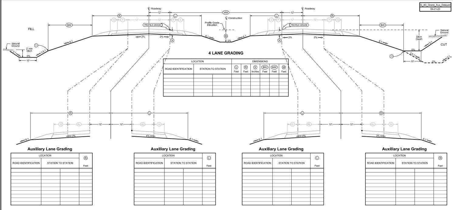
Normal section shown may be modified appropriately in areas of superelevated curves or other locations specifically designated by the Engineer.
