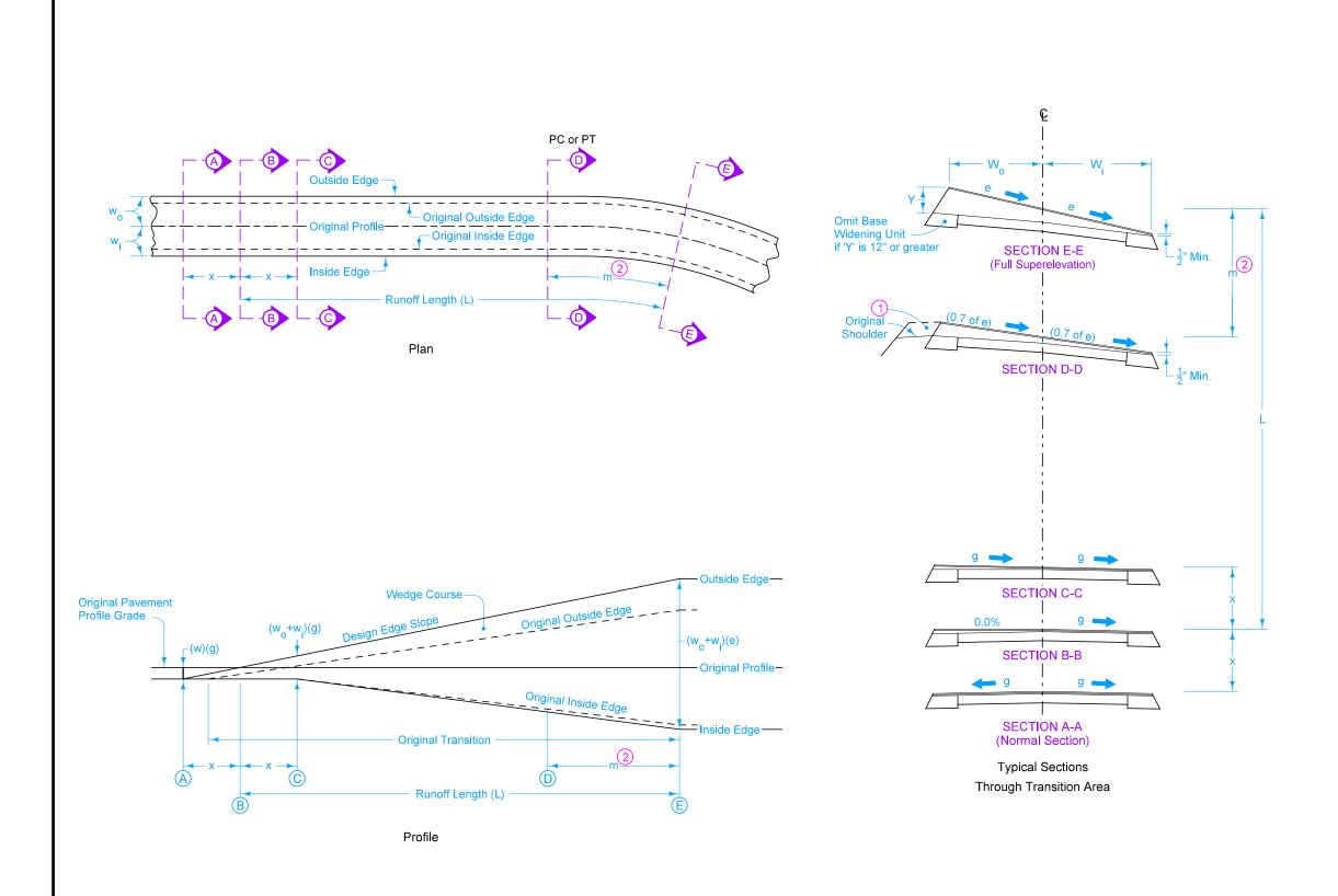
Refer to curve data contained in the project plans for tangent runout length (x), runoff length (L), transition applied within curve length (m), rotation width (w), total thickness of wedge and surface mat (Y), normal cross-slope (g), existing cross slope at PC/PT (E), and full superelevation (e).
