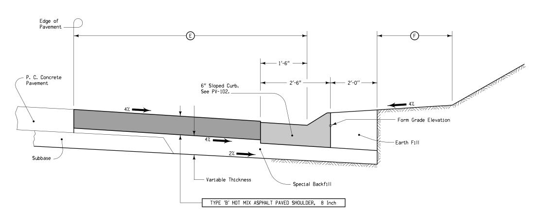
TYPICAL SECTION HOT MIX ASPHALT PAVED SHOULDER WITH 6" SLOPED CURB AND GUTTER UNIT
