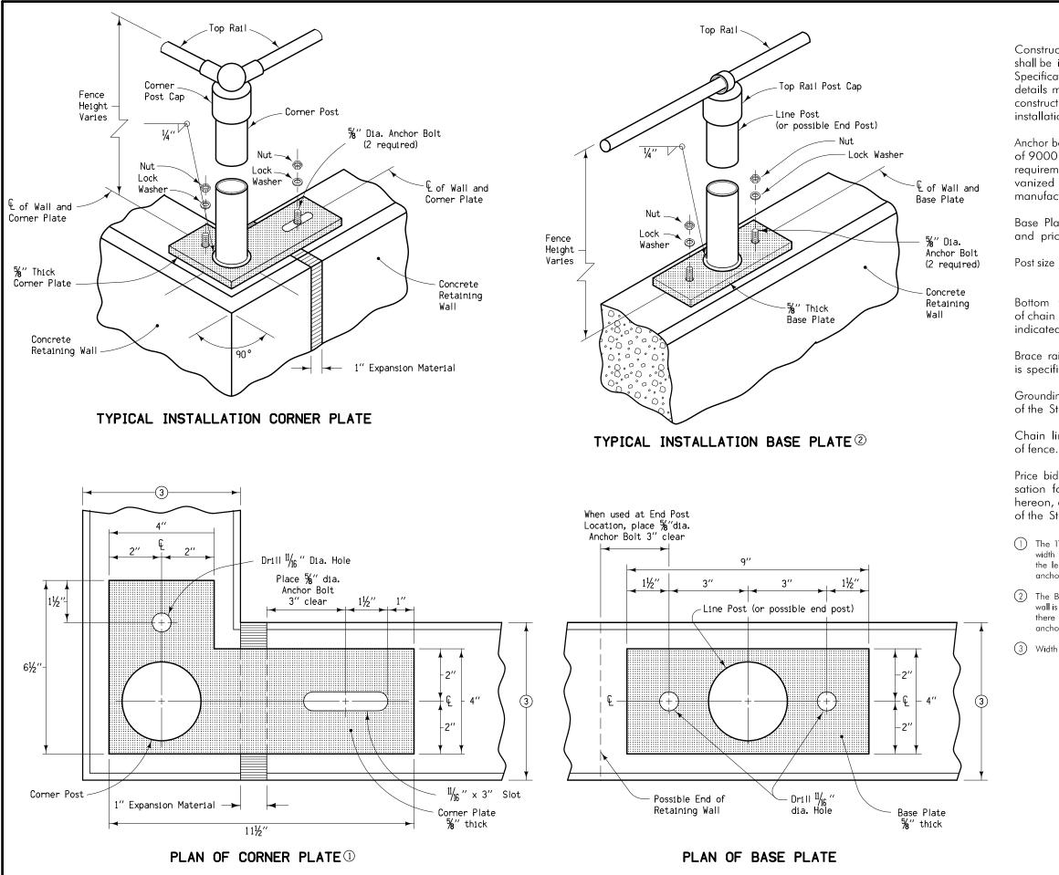
Construction of Chain Link Fence on Concrete Retaining Wall shall be in conformance with current Standard and Supplemental Specifications. Details shown on this sheet are typical. Alternate details may be submitted to the Engineer for approval prior to construction. Refer to project plans for details of particular fencing installations.
