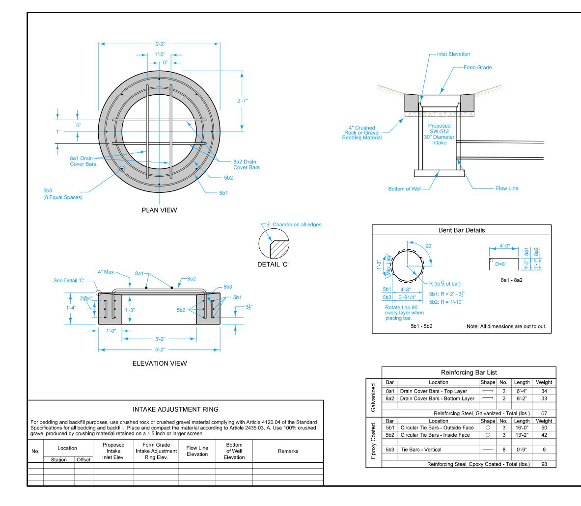
Minimum clear distance of 3 inches from the face of concrete to near reinforcing bar unless noted otherwise.
