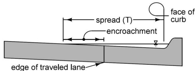
**Figure 1:** Curb section showing spread and encroachment.
