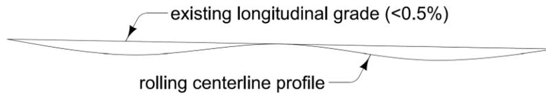
**Figure 1:** Rolling centerline profile.
