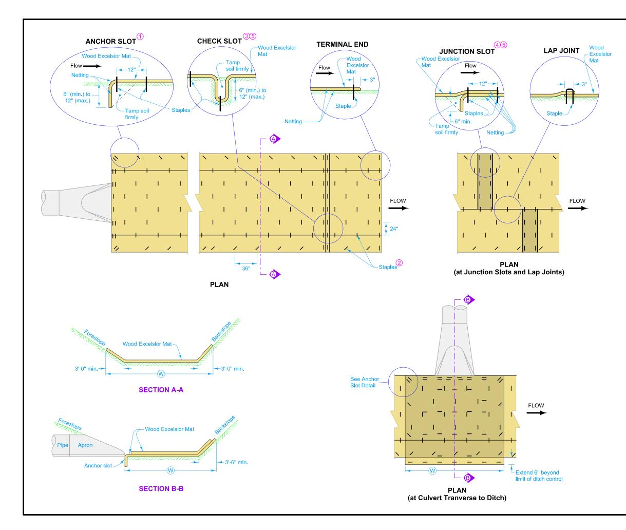
Provide necessary excavation at locations where silt conditions require shaping of a ditch to provide a proper type of area for installation of wood excelsior mat for special ditch control.
