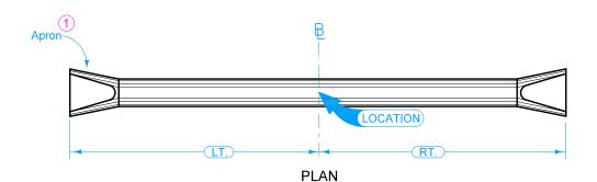
Skew angle is the angle which one end of the pipe is ahead (by stationing) of line perpendicular to the  ${\bf L}$ . (Example: skew Rt. ahead 30 degrees)
