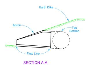
Use when specified. This type of inlet assembly may be substituted for the inlet apron shown on drawings of standard type drainage structures
