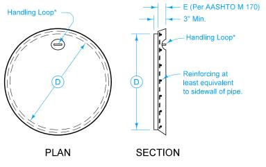
\*The handling loop may be omitted when the cap is placed in a buried installation.
