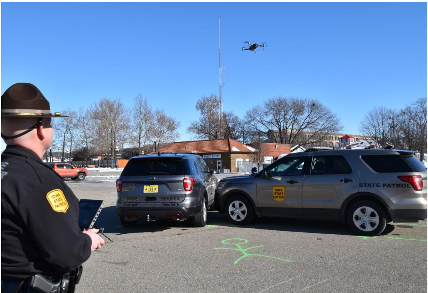
State Trooper Mark Anderson pilots the sUAS over the mock crash site, taking pictures to create a 3-D model of the scene.
