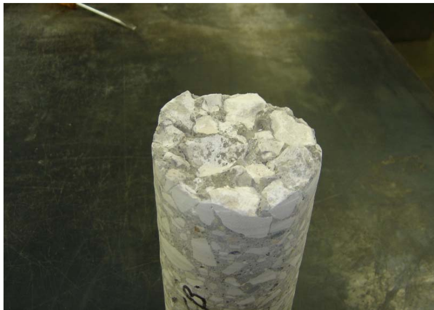
Figure 3. Concrete core with granular subbase removed.
