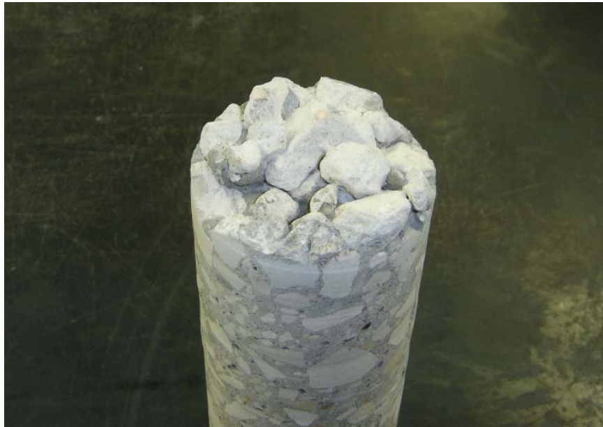
Figure 2. Concrete core with granular subbase attached.
