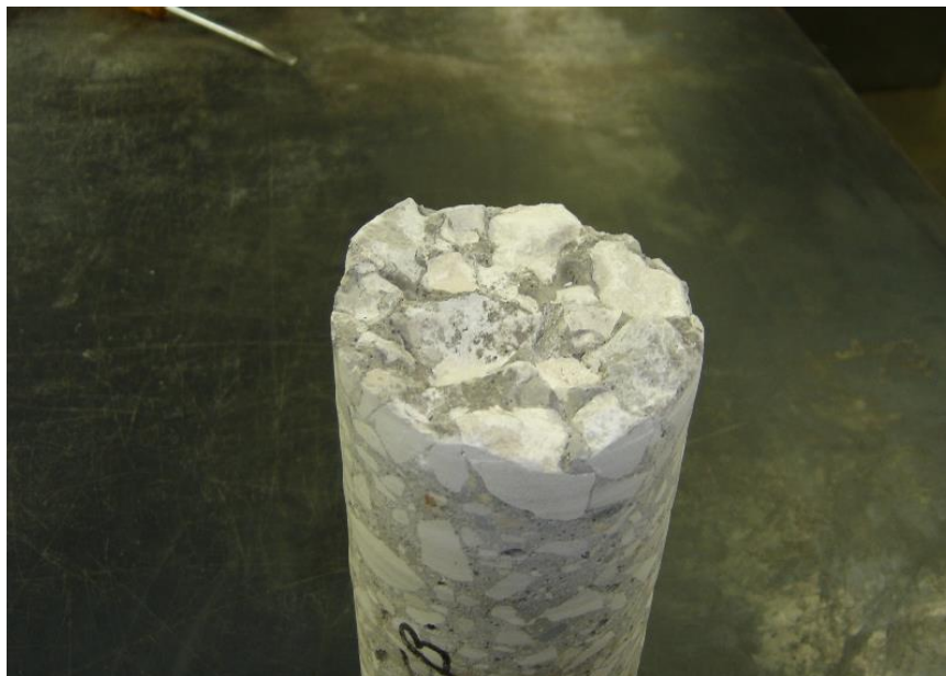
Figure 3. Concrete core with granular subbase removed.
