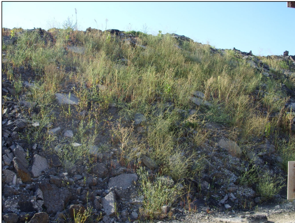
Figure 2. Recycled stockpile contaminated with organic material.
