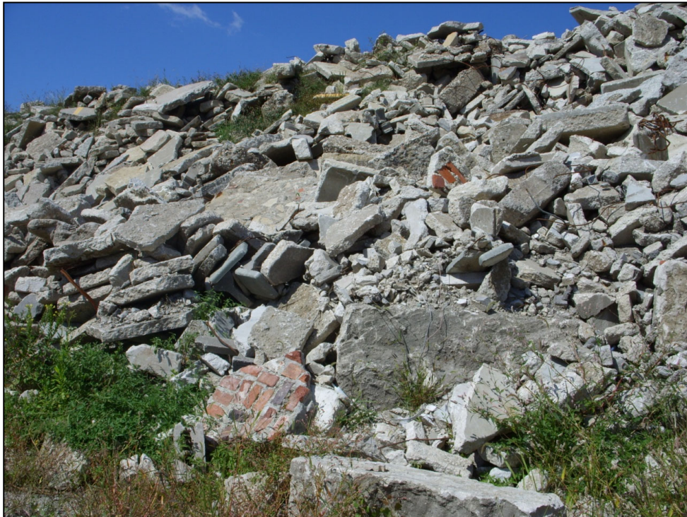
Figure 4. Recycled stockpile contaminated with non-pavement material.
