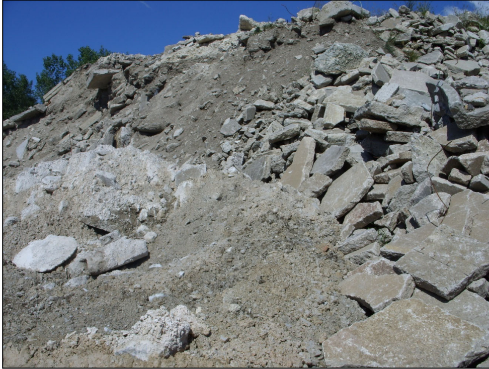
Figure 3. Recycled stockpile with excessive fines.
