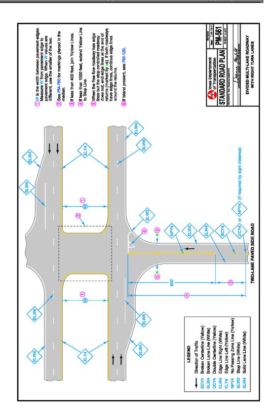
Figure 18b Standard Road Plan PM-561 Link
