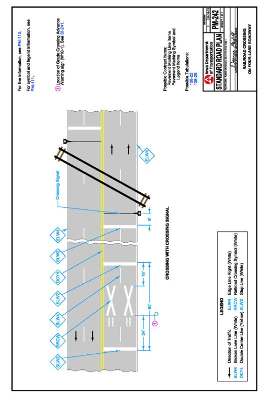
Figure 10 Standard Road Plan PM-242 Link
