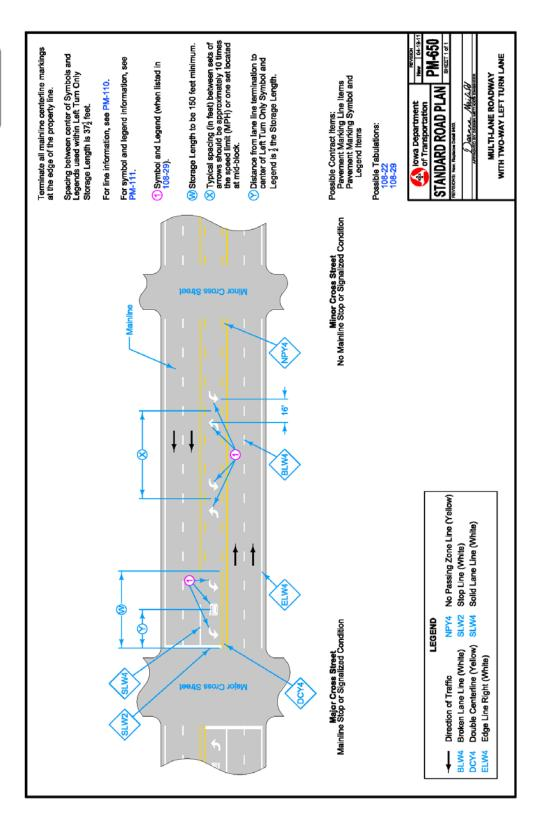
Figure 21 Standard Road Plan PM-650 Link
