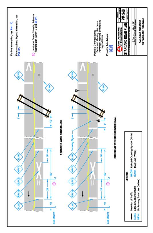
Figure 9 Standard Road Plan PM-240 Link
