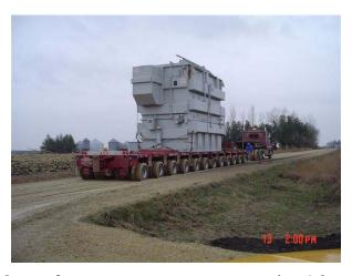
Figure 3.12. Electrical transformer en route to power station (photo courtesy of Mitchell County)
