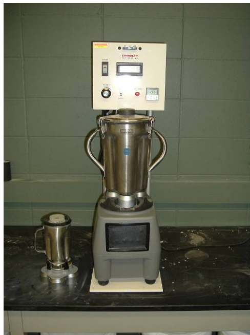
Figure 8. Chandler Engineering Waring Blender
