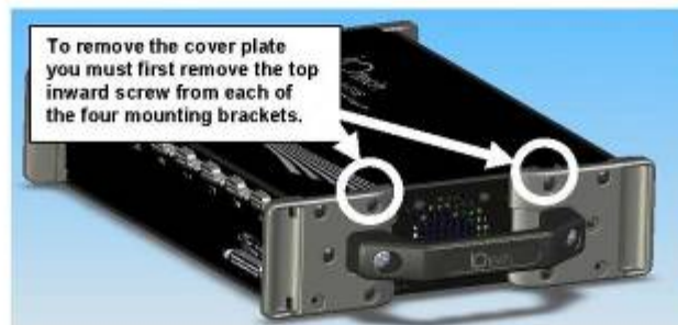
The Cover Plate Is Secured by 4 Screws [2 Screws per side]
