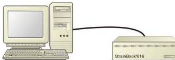
Connecting a StrainBook/616 to the Ethernet
