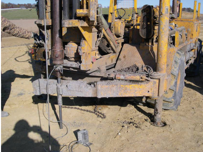
Figure 56. CPTU testing conducted at STA 143+50 westbound Crow Creek embankment on 10/31/06
