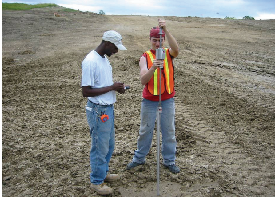
Figure 21. DCP testing conducted by ISU research team
