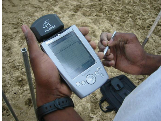
Figure 7. G-RAD system with GPS attachment on a Dell pocket PC
