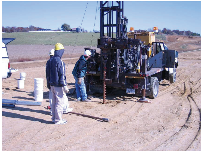
Figure 57. ISU soil boring at STA 143+50 westbound Crow Creek embankment on 10/31/06
