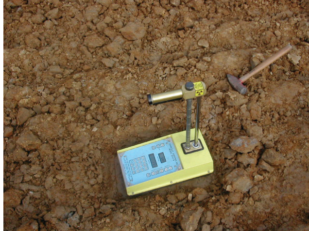
Figure 4. Humboldt nuclear moisture-density gauge
