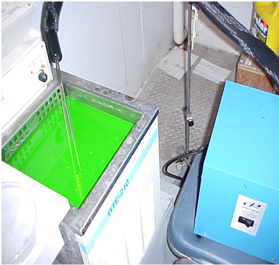
1. Cooling bath-chiller unit and thermistor
