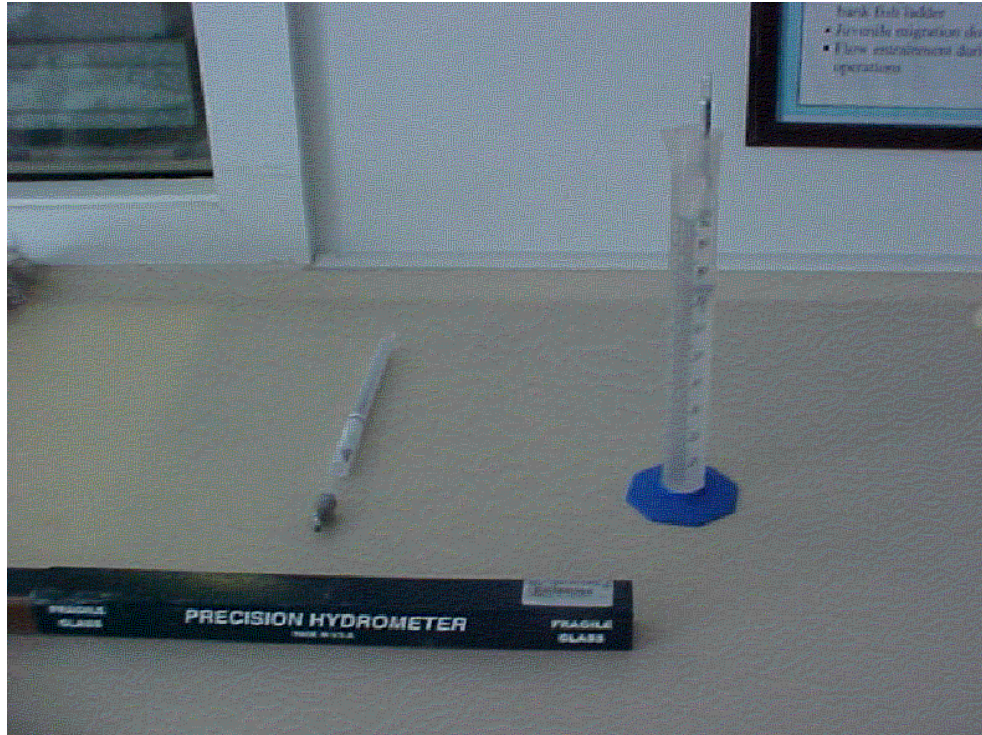
Figure 3.5: Specific gravity is measured using a hydrometer
