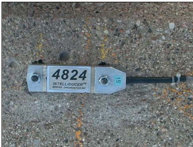
Figure 6.6. A BDI strain transducer
