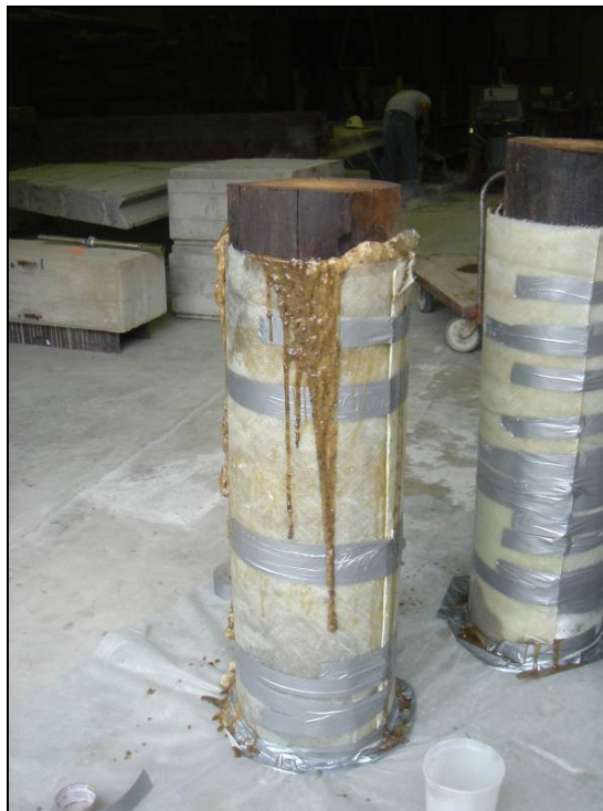
Figure 13.14. Expandable wood filler epoxy applied to fill the void between the pile and the FRP shell
