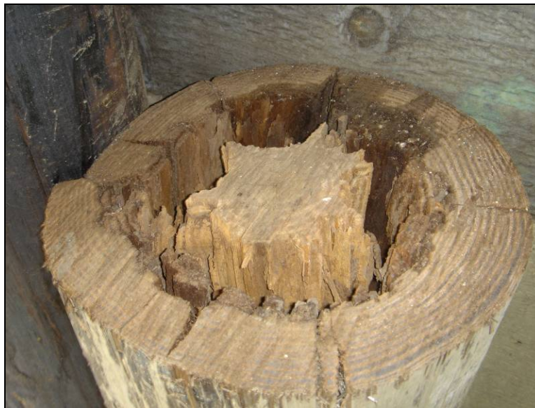
Figure 5.1. Significant internal pile deterioration that is difficult to detected using the stress wave technique (Bridge No. 31-72-50 Tama County – June 10 2005)
