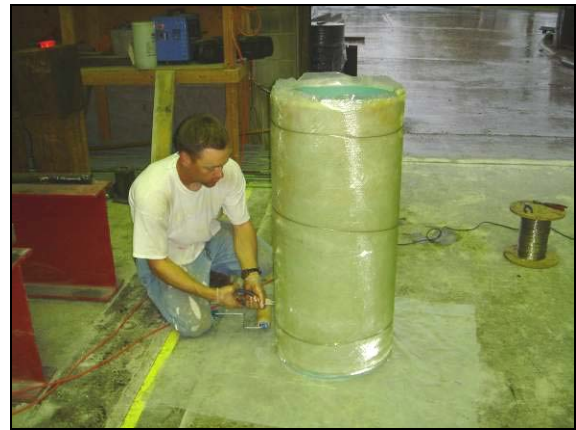
(b) FRP sheets wrapped around the pipe
