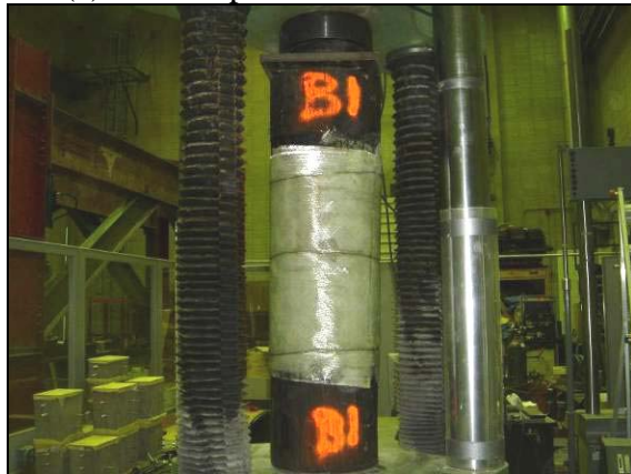
(c) Repair method B – axial
