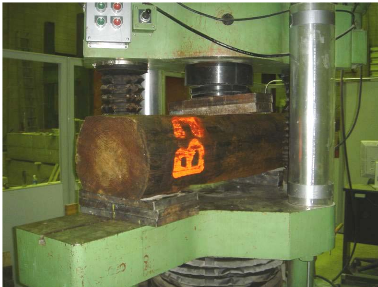
Figure 13.3. Pile sides flattened for conducting bending tests
