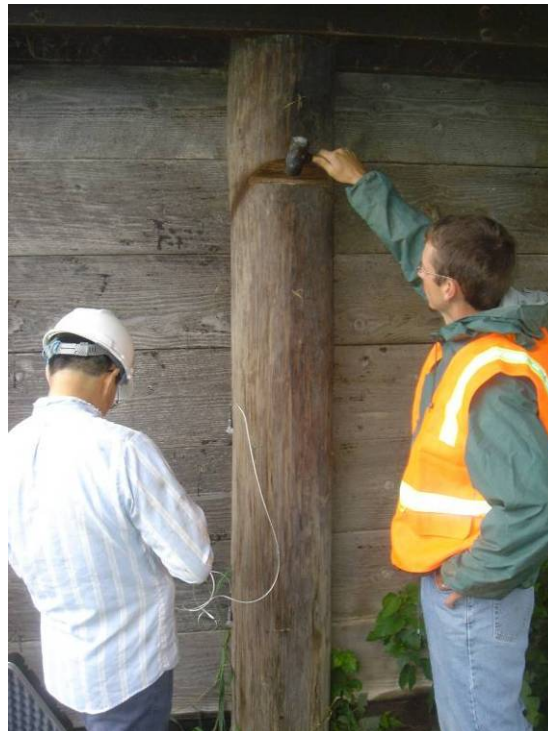
Figure 9.24. Applying an axial impact to the notched pile (Bridge No. 237350 Mahaska County – August 17 2006)
