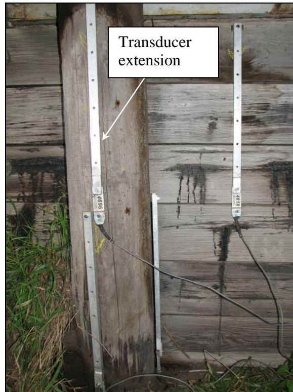
Figure 6.7. A BDI strain transducer with an extension (Bridge No. 02-90-70 Humboldt County – July 10 2006)
