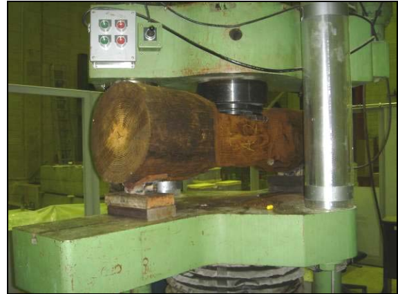
(b) Control pile section – bending
