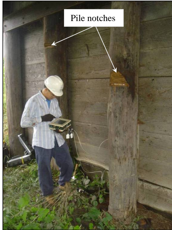
Figure 9.23. Notches created in the exposed piles to allow for axial impact (Bridge No. 237350 Mahaska County – August 17 2006)
