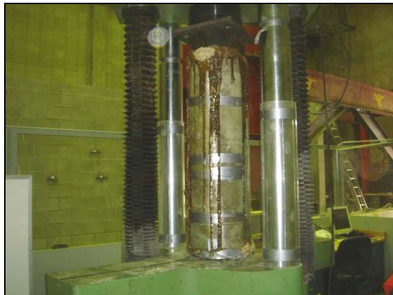
(e) Repair method C – axial
