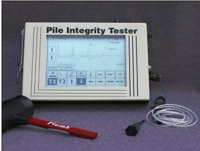
Figure 9.21. Equipment used in Pile Integrity Testing
