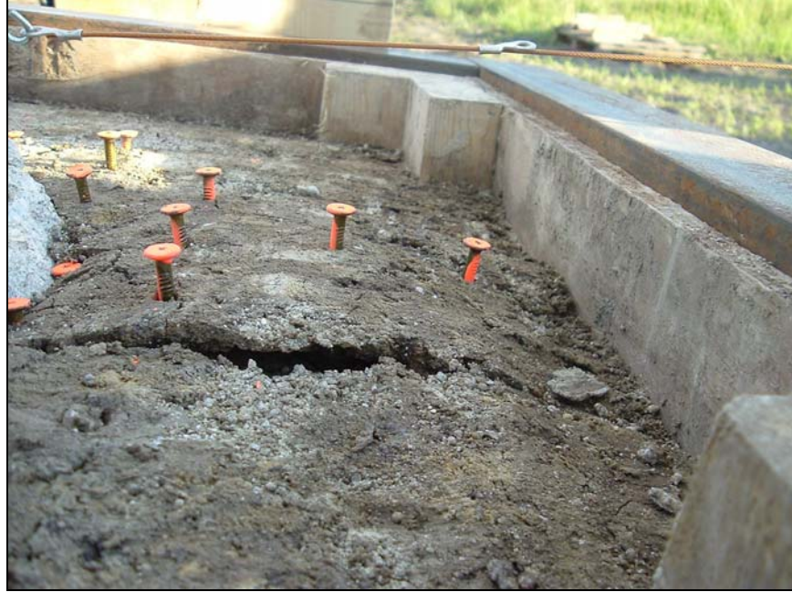
Figure 111. Soil bulging behind pile (115-mm Pile in glacial till)
