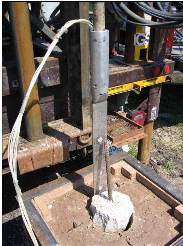
Figure 109. K_0 stepped blade test performance
