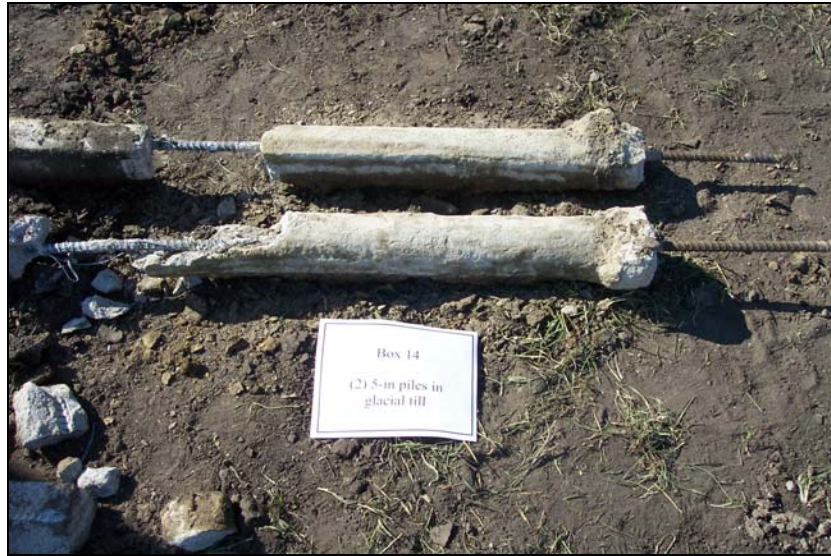
Figure 121. Exhumed 127-mm piles (Pile 14 A and 14 B)
