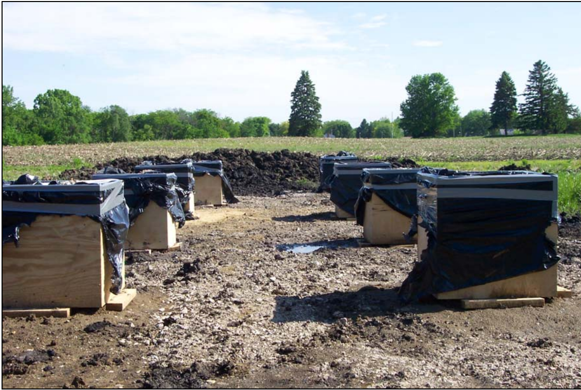
Figure 36. Prepared shear box forms
