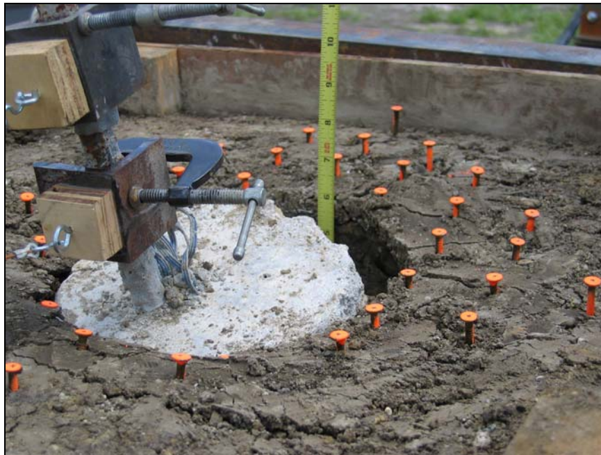
Figure 110. Gap in front of pile (115-mm Pile in glacial till)
