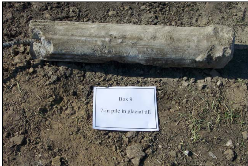
Figure 120. Exhumed 178-mm pile (Pile 9)
