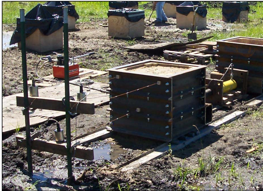
Figure 40. Displacement gauge locations on shear boxes
