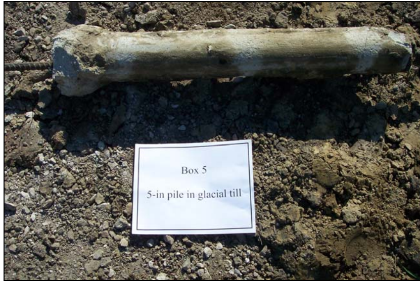
Figure 119. Exhumed 127-mm pile (Pile 5)
