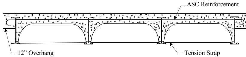
Figure 1.2. Cross section with the transverse arch implemented.
