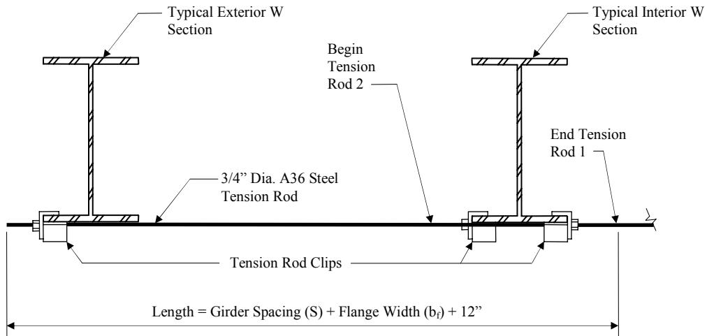
Figure 5.10. Typical layout of the tension rods and clips.
