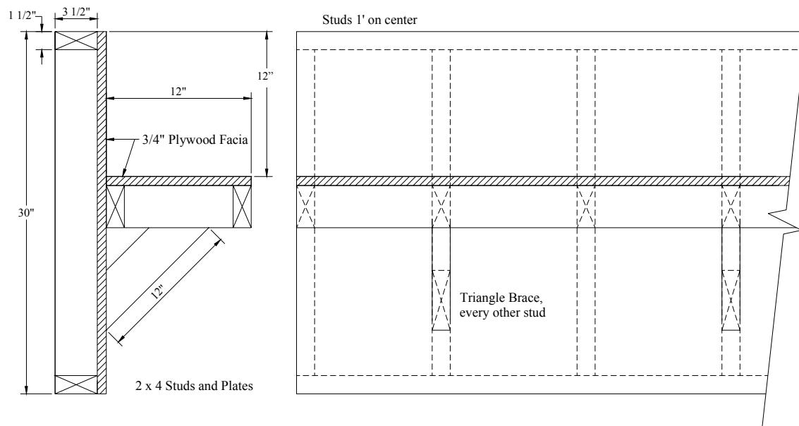
Figure 5.4. Typical exterior formwork panel used for MBISB 2.
