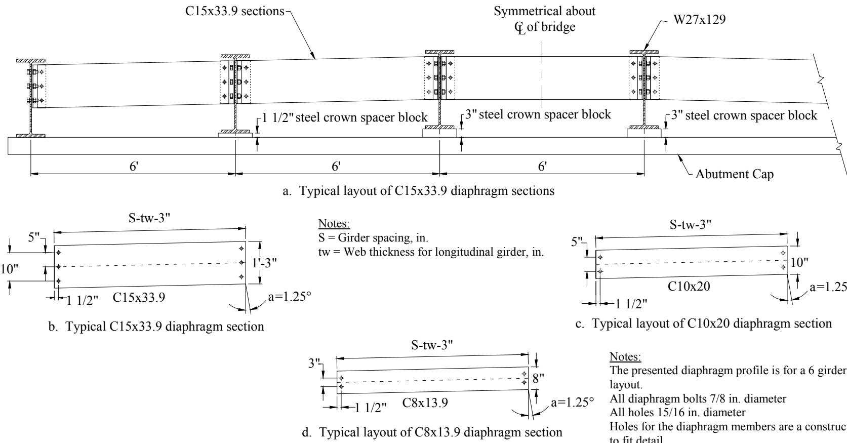
Figure 4.5. Profile of the suggested diaphragm system for the MBISB design.
