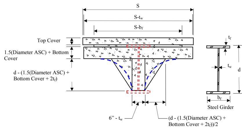
b. Detail A: Approximated interior cross section
