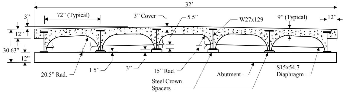
Figure 3.6. Cross section of MBISB 2.
