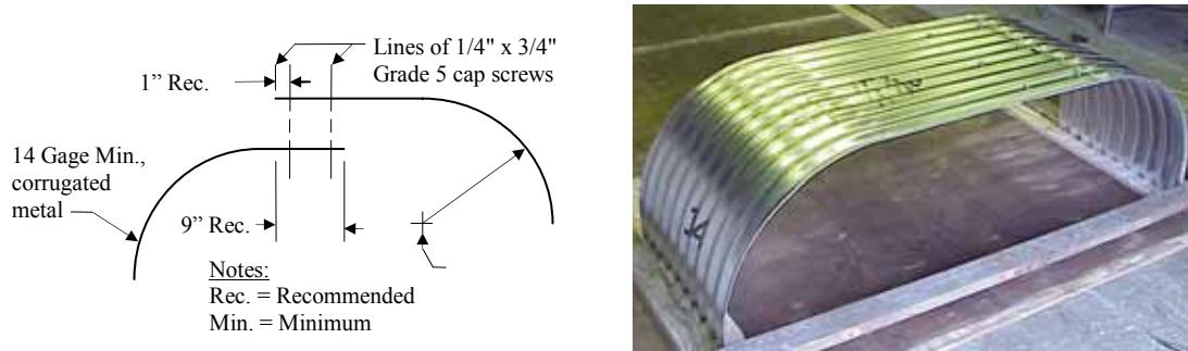
a. Exploded view of circular arched formwork section      b. Completed arched formwork section
