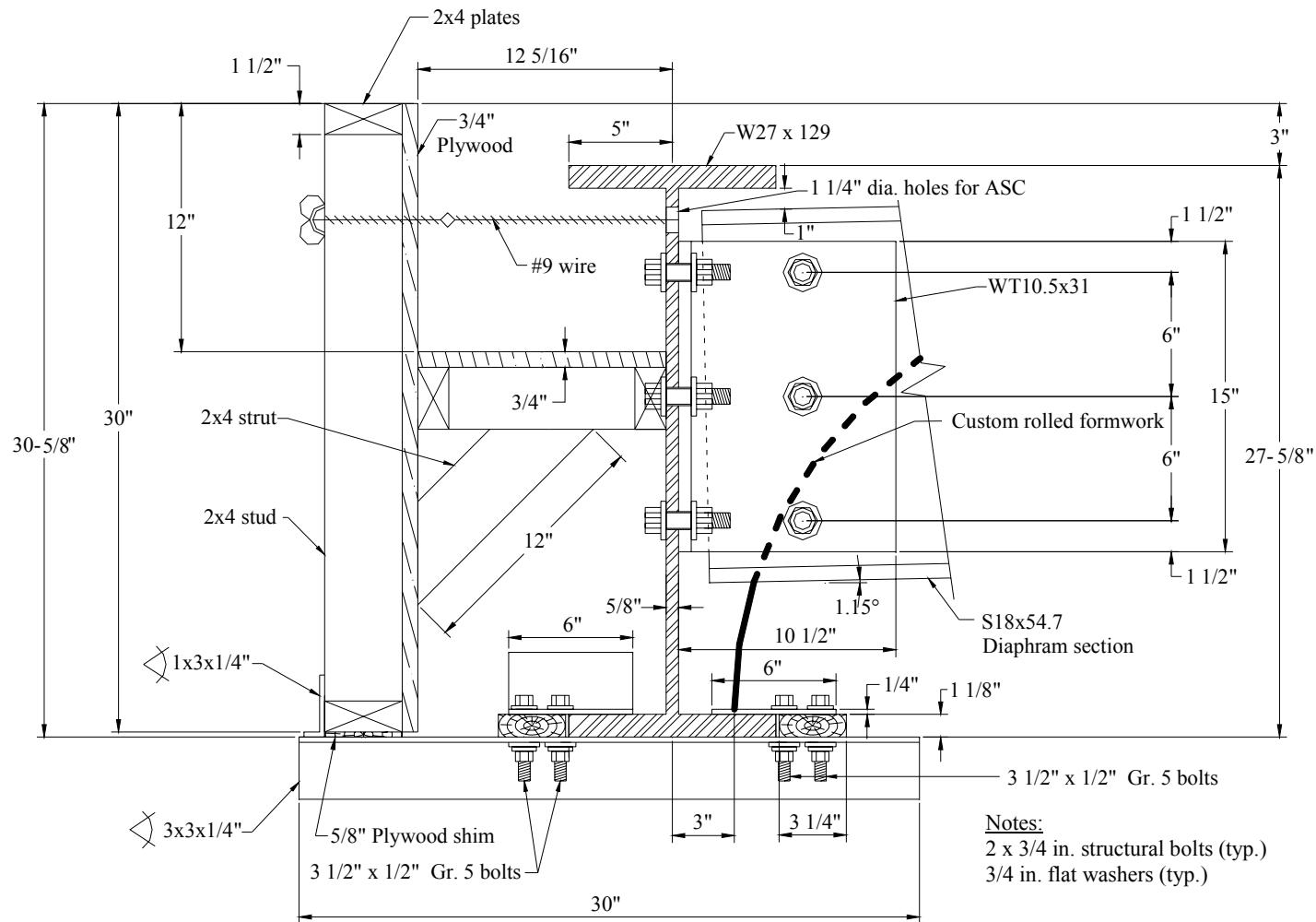
Figure 5.5. Installed exterior formwork.
