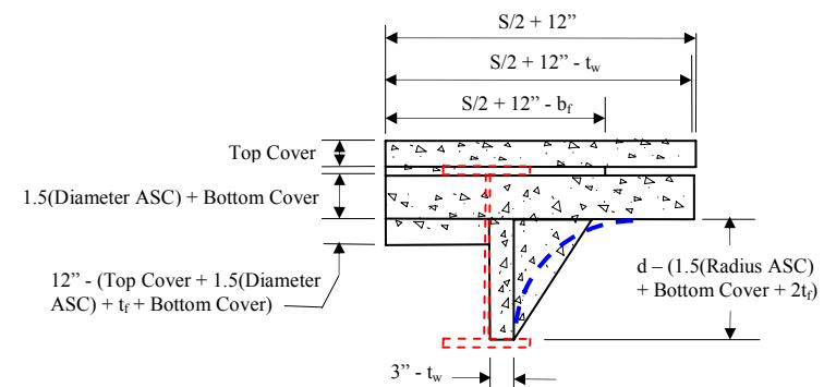
c. Detail B: Approximated exterior cross section
