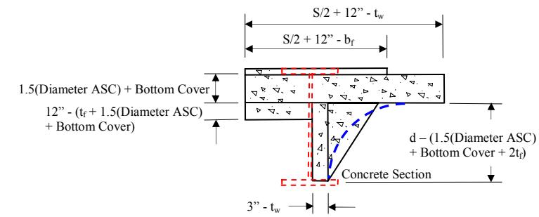
(c) Detail B: Approximated exterior cross section
