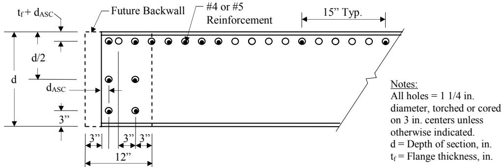
Figure 4.12. Layout of deck reinforcement.
