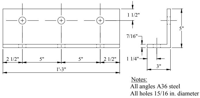
a. Diaphragm connector for C15x33.9 section
