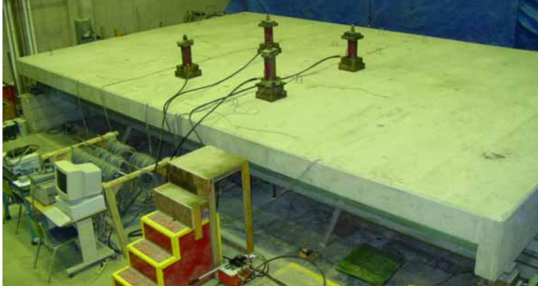
c. Over view of the model bridge during the ultimate flexural loading
