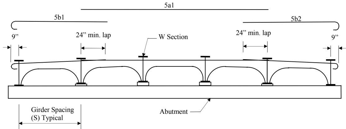
Figure 5.6. Transverse reinforcement for the MBISB design.
