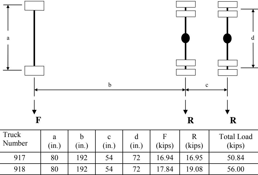
Figure 3.8. Wheel and load configurations of the MBISB 2 test vehicles.
