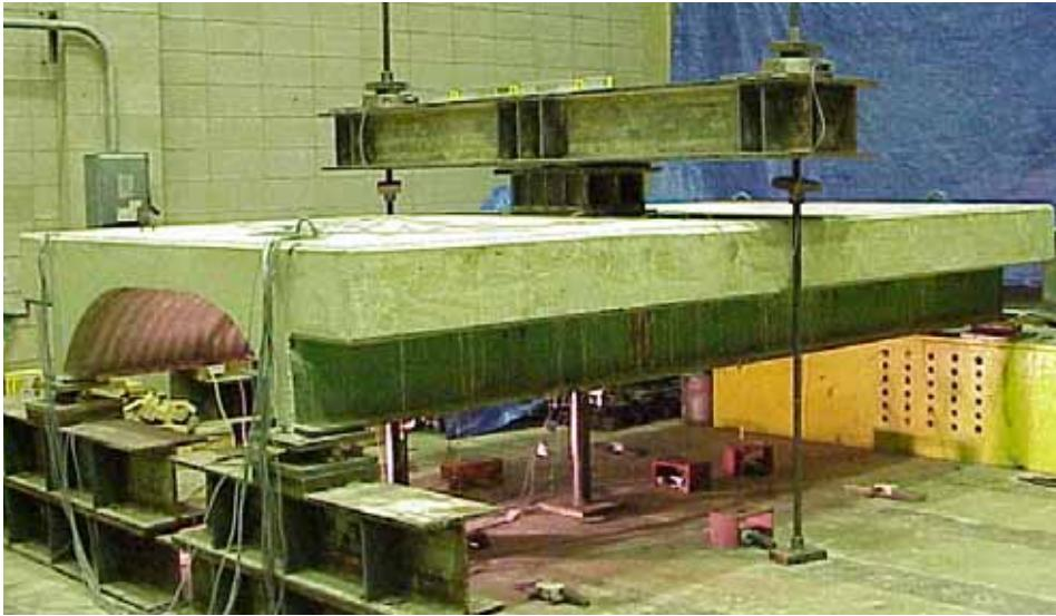
Figure 2.2. Typical setup of the ultimate punching shear test for a single bay specimen.
