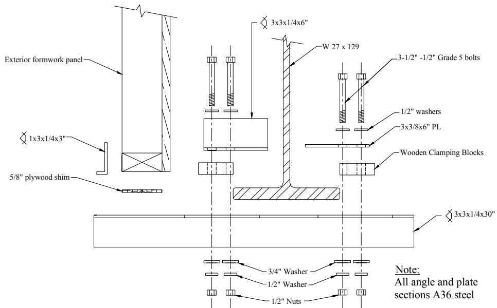
a. Exploded view of the exterior formwork support
