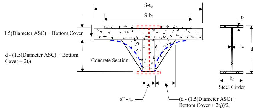
(b) Detail A: Approximated interior cross section
