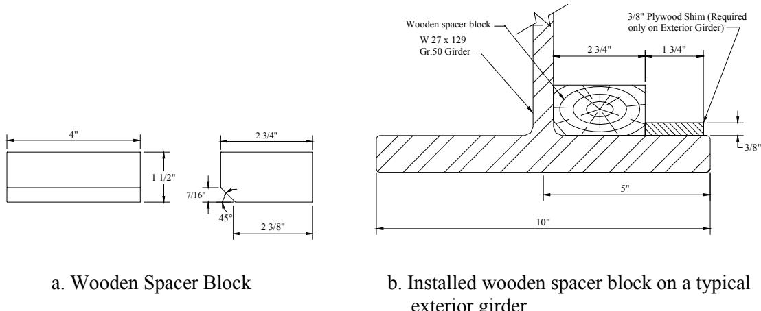
Figure 5.2. Wooden spacer block for securing the custom rolled arched formwork.
