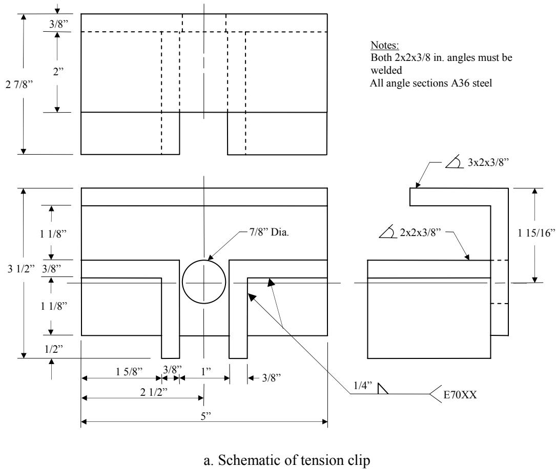
a. Schematic of tension clip
