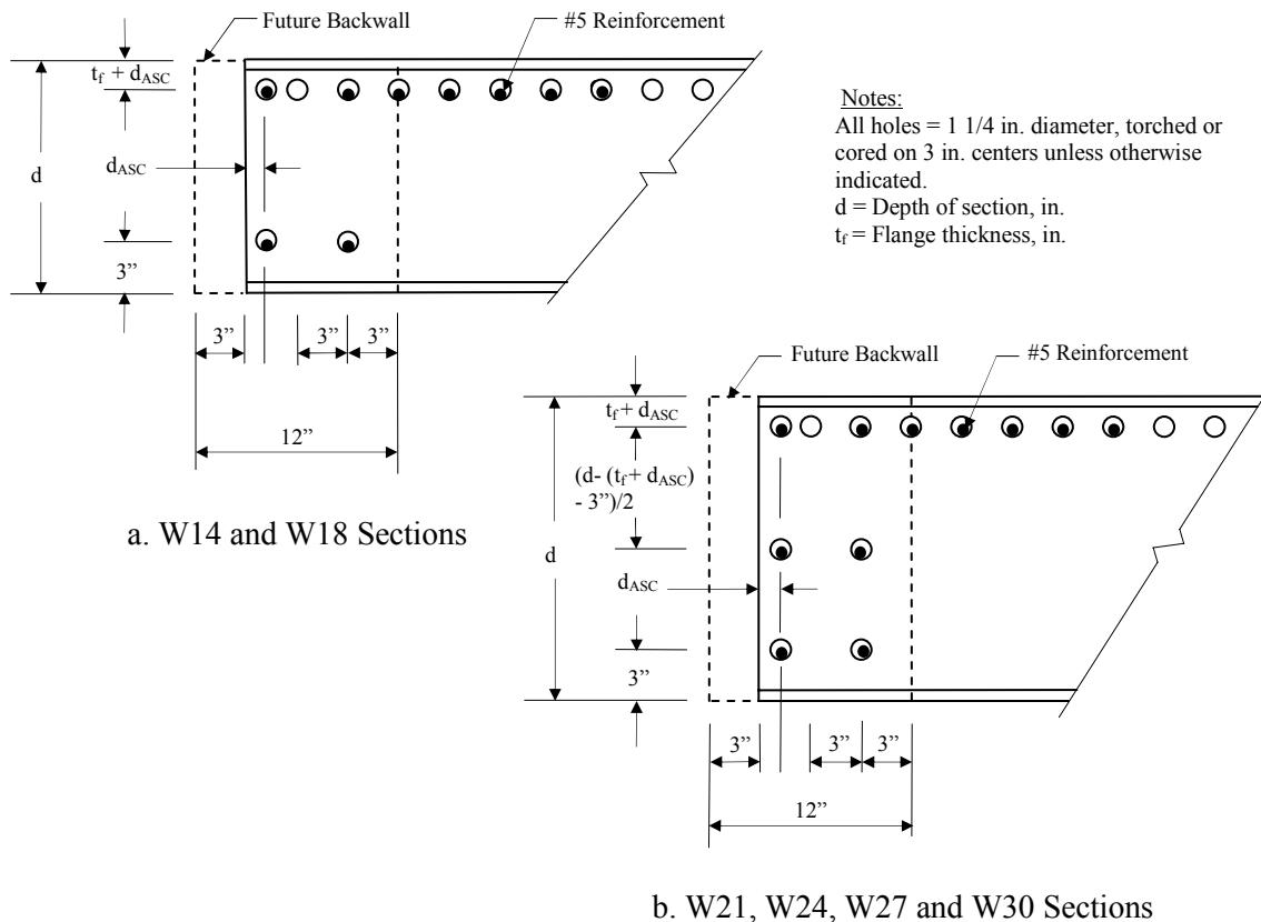
Figure 4.6. Layout of backwall reinforcement for future MBISBs.
