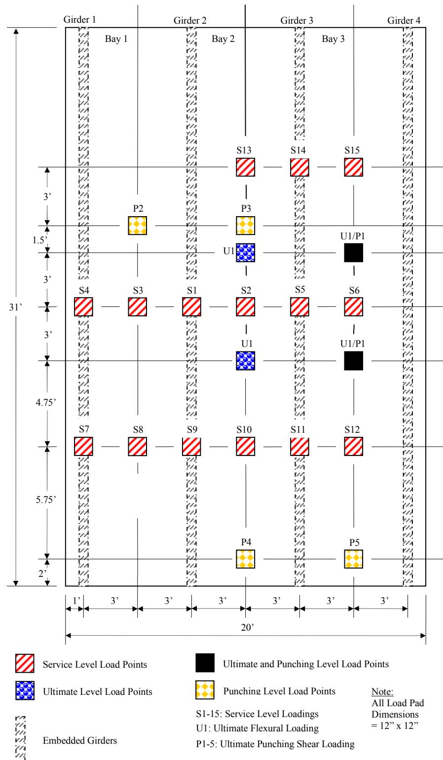
Figure 2.4. Plan view of model bridge illustrating various load points.
