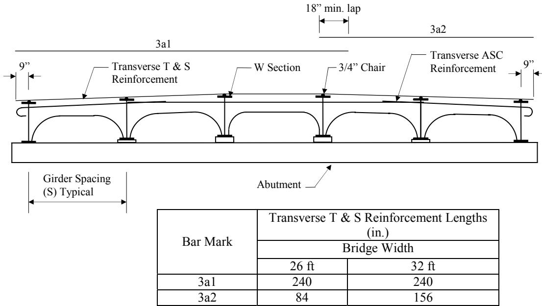
Figure 5.9. Layout of transverse T & S reinforcement.
