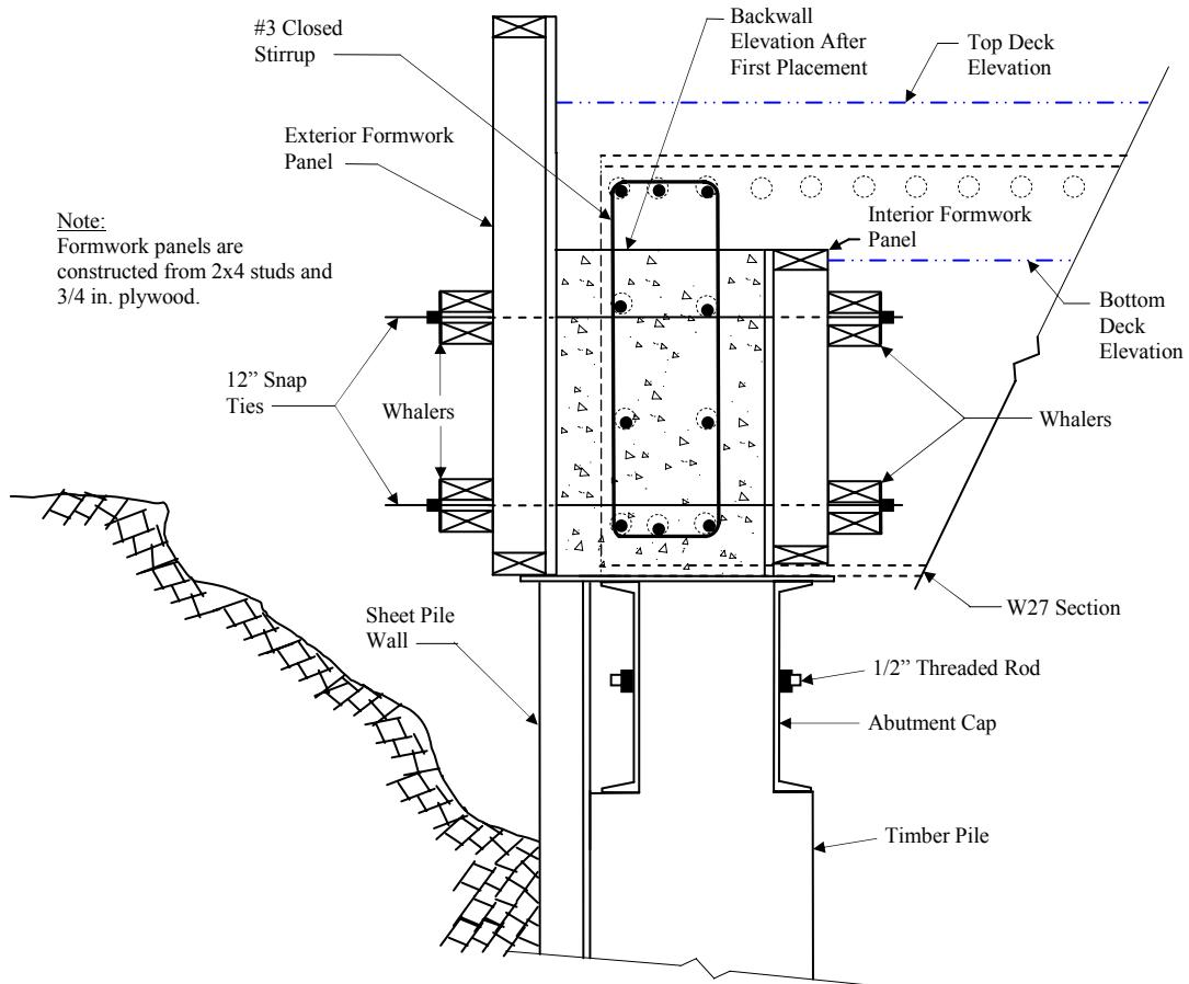
a. Cross section of backwall formwork
