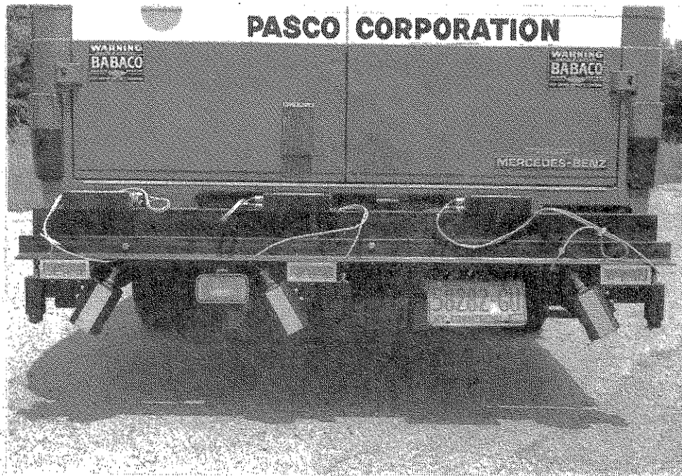
Fig. B.14. Laser mounting on PASCO vehicle.
