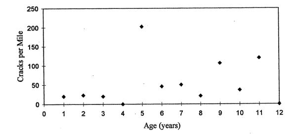
Figure 6: Frequency of transverse cracking
