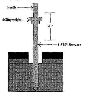
**Figure 14: Dynamic Cone Penetrometer**
