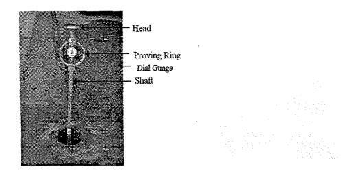
**Figure 13. Soil Cone Penetrometer**
