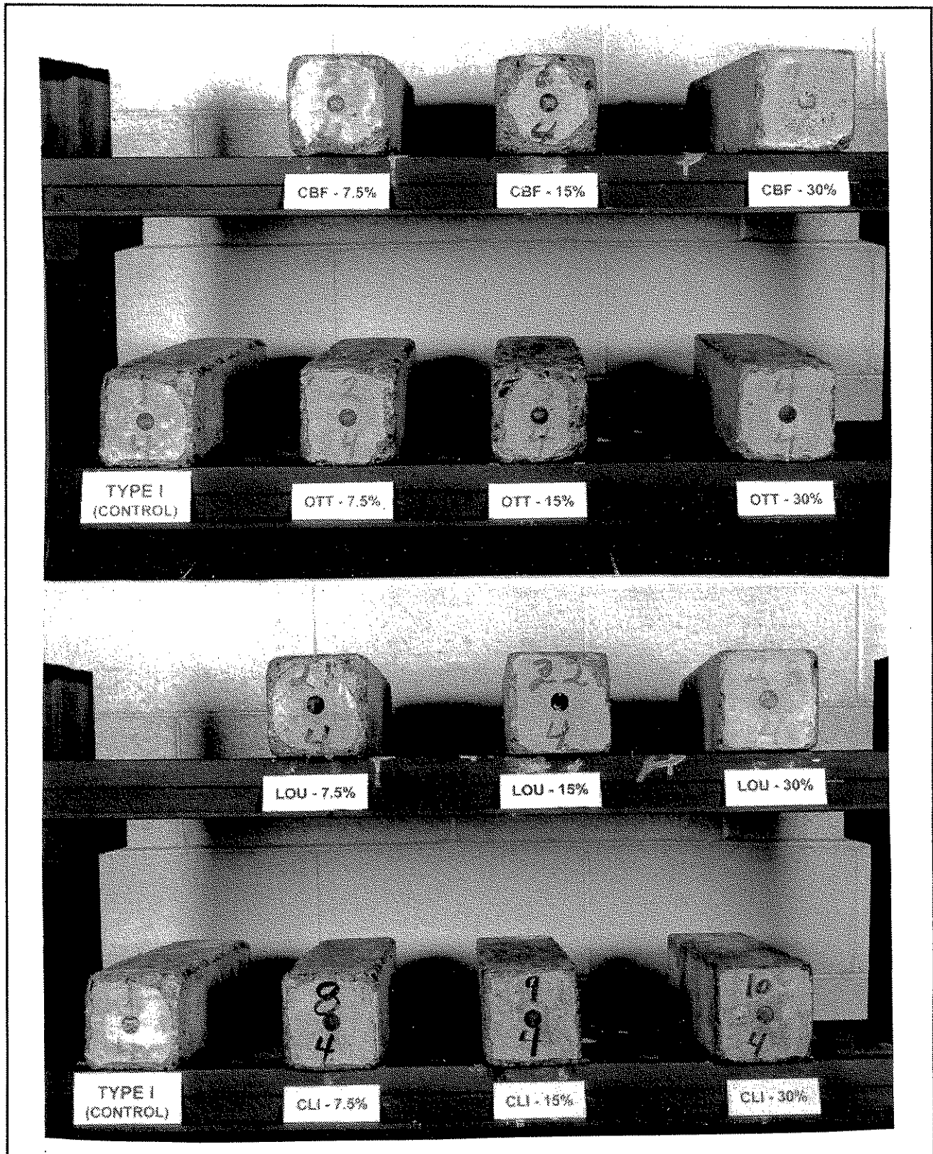
Figure 20. Specimens subject to the 10 percent sulfate soak test; Type I cement, various fly ashes at 7.5, 15 and 30 percent replacement, Jaben aggregate, age about 128 weeks.
