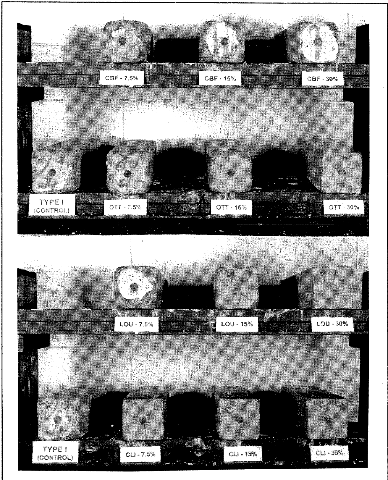
Figure 22. Specimens subject to the 10 percent sulfate soak test; Type I cement, various fly ashes at 7.5, 15 and 30 percent replacement, Early Chapel aggregate, age about 64 weeks.
