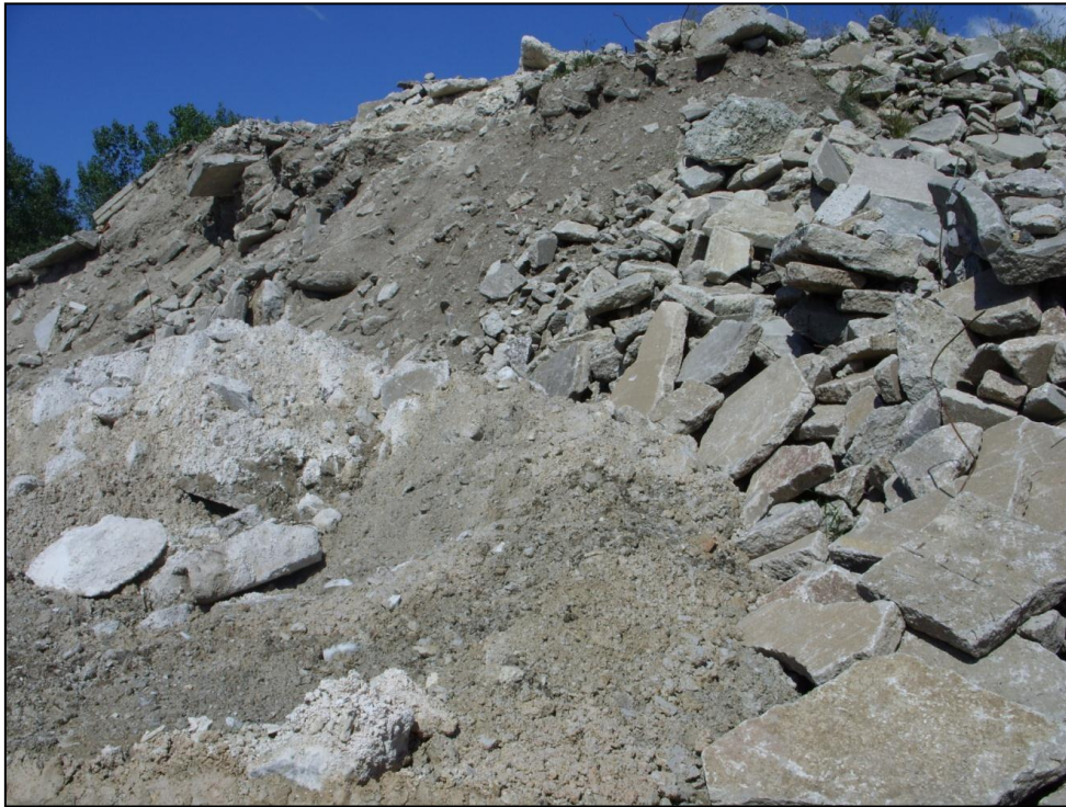
Figure 3. Recycled stockpile with excessive fines.
