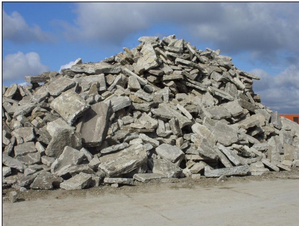
Figure 6. Example of a clean stockpile of recycled PCC.
