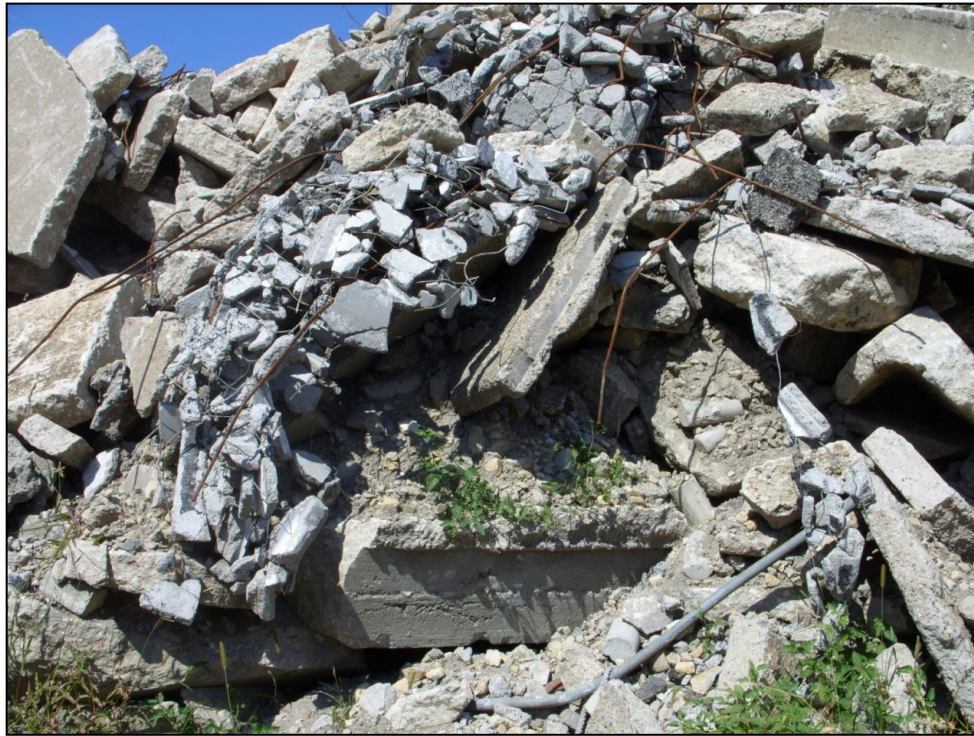
Figure 1. Recycled stockpile contaminated with steel.
