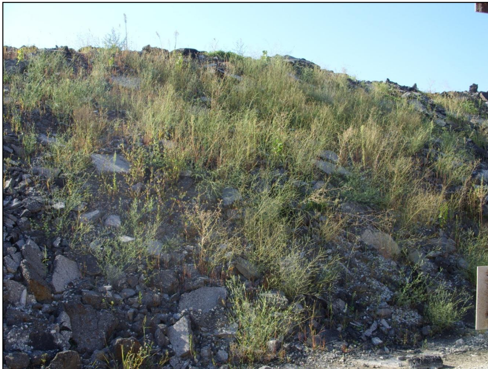
Figure 2. Recycled stockpile contaminated with organic material.
