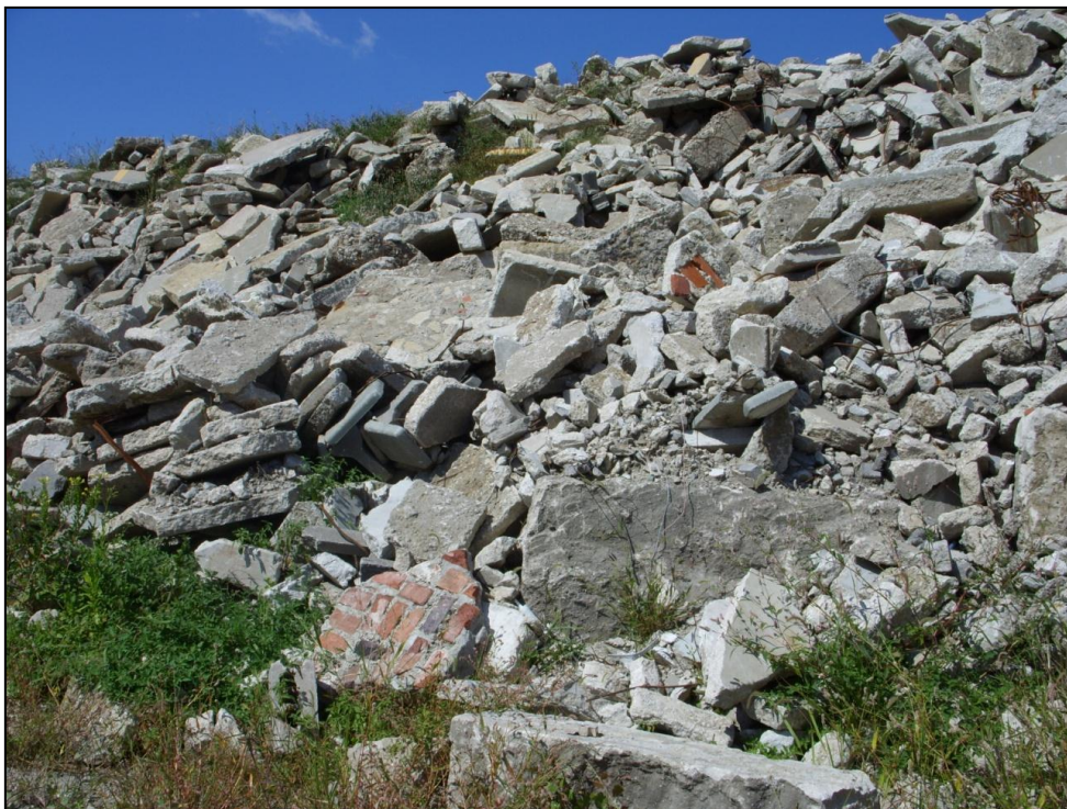
Figure 4. Recycled stockpile contaminated with non-pavement material.
