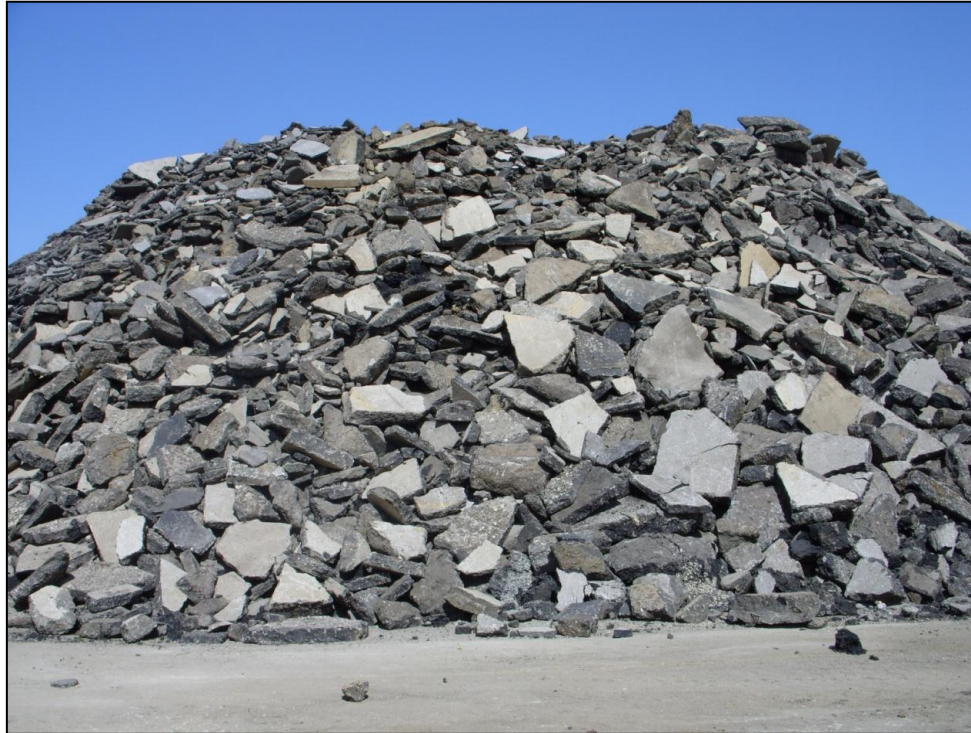
Figure 5. Example of a clean stockpile of recycled HMA.
