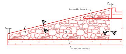
Typical Wingwall Elevation
