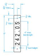
DELINEATOR REFERENCE POINT PLAQUE Place delineators at a constant distance from the edge of traveled way and/or the edge of shoulder.
